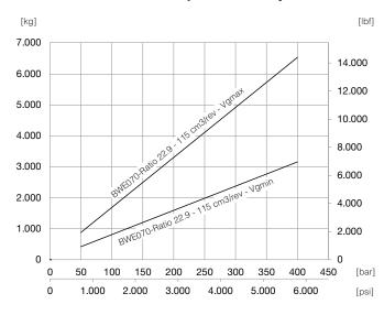
$Vg_{max} = 115 \text{ cm}^3/\text{rev} [7.00 \text{ in}^3/\text{rev}]$  $Vg_{min} = 56 \text{ cm}^3/\text{rev} [4.40 \text{ in}^3/\text{rev}]$
