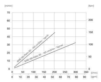
$Vg_{max}$  = 166.2 cm³/rev [10.13 in³/rev] - Max 300 l/min [79 gpm] allowed  $Vg_{min}$  = 80 cm³/rev [4.88 in³/rev] - Max 201 l/min [53 gpm] allowed
