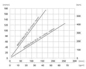
$\label{eq:Vg_max} Vg_{max} = 85\ cm^3/rev\ [5.17\ in^3/rev] - Max\ 255\ l/min\ [67\ gpm]\ allowed \\ Vg_{min} = 40\ cm^3/rev\ [2.43\ in^3/rev] - Max\ 166\ l/min\ [44\ gpm]\ allowed \\$
