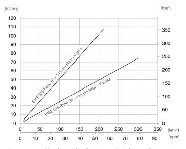
Vg<sub>max</sub> = 115 cm<sup>3</sup>/rev [7.05 in<sup>3</sup>/rev] - Max 300 l/min [80 gpm] allowed Vg<sub>min</sub> = 56 cm<sup>3</sup>/rev [3.416 in<sup>3</sup>/rev] - Max 212 l/min [56 gpm] allowed
