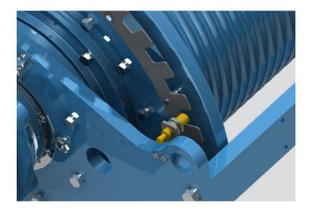
Our stainless-steel Proximity sensor is used to read the rotational speed of the drum, providing the user an information of the rope speed. Using two sensors is also possible to define the sense of rotation of the drum, giving information about lifting or lowering of the load.
