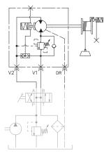
The supply, return and drain hoses must all be of adequate internal dimensions to support the maximum working and drainage flow rates. Draining hoses must always flow directly to the oil reservoir.
