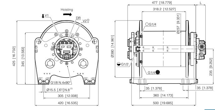
$^{(1)}$  As Standard with single overcenter valve, double overcenter valve available on request.  $^{(2)}$  N. 8 bolts for ABS certified version only. N. 4 bolts for other versions.
