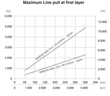
Vg<sub>max</sub> = 85 cm<sup>3</sup>/rev [5.17 in<sup>3</sup>/rev] Vg<sub>min</sub> = 40 cm<sup>3</sup>/rev [2.43 in<sup>3</sup>/rev]
