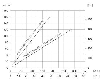
Vg<sub>max</sub> = 115 cm<sup>3</sup>/rev [7.00 in<sup>3</sup>/rev] - Max 290 l/min [76 gpm] allowed Vg<sub>min</sub> = 56 cm<sup>3</sup>/rev [4.40 in<sup>3</sup>/rev] - Max 183 l/min [48 gpm] allowed
