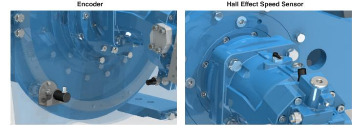
The Encoder reads the speed of the drum and the rotation direction, providing information on the speed of the rope. Using an absolute encoder is also possible to collect information about the length of the rope still on the drum or unwounded. It is also possible to have the rotative speed sensor on the Brevini<sup>®</sup> Hydraulic Motor.
