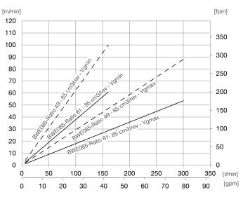
$Vg_{max}$  = 85 cm³/rev [5.18 in³/rev] - Max 300 l/min [80 gpm] allowed  $Vg_{min}$  = 40 cm³/rev [2.44 in³/rev] - Max 160 l/min [43 gpm] allowed
