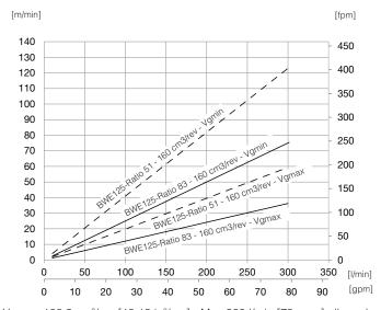
$Vg_{max} = 166.2 \text{ cm}^3/\text{rev} [10.13 \text{ in}^3/\text{rev}] - Max 300 \text{ l/min} [79 \text{ gpm}] allowed Vg_{min} = 80 \text{ cm}^3/\text{rev} [4.88 \text{ in}^3/\text{rev}] - Max 300 \text{ l/min} [79 \text{ gpm}] allowed$
